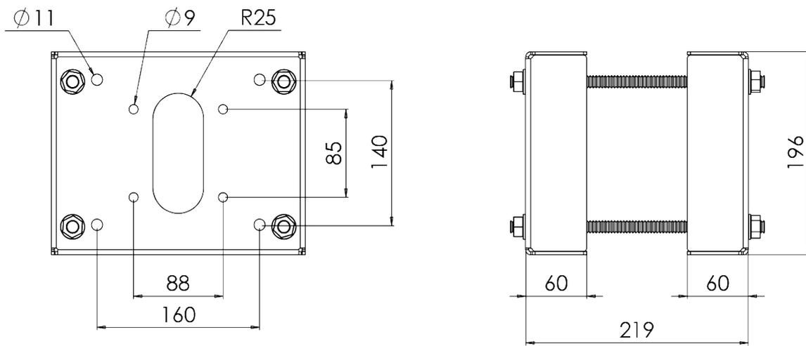
SSPM129LC/SSPM168/SSPM168LC/SSPM204/SSPM250/SSPM254 orthographic views
