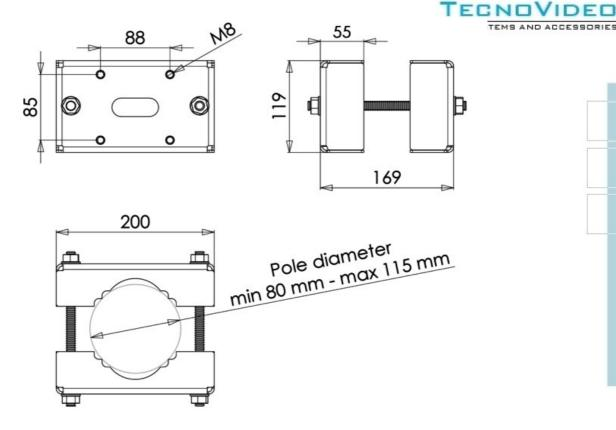
SSPM101/SSPM129/SSPM129AC orthographic views
